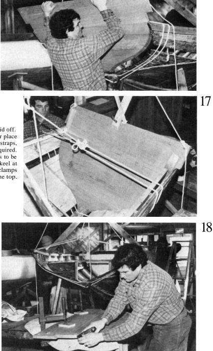
All the careful measuring and cutting has paid off. After the hull has been pulled into its proper place against the new transom and held there with straps, braces, and clamps, very little trimming is required. At this stage, before fastening, the transom has to be held aft with a block of wood clamped to the keel at the bottom, and with wedges against the sheer clamps at the top.
