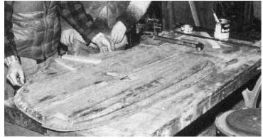
But not all 12 1/2-footer transoms are exactly alike, and differences from boat to boat show up when the old transom is laid on the master pattern. In most cases, the stripped-out hull can be pushed and pulled a little to conform to the pattern, since differences seldom amount to more than 1/4".
