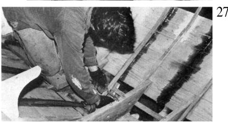
Once its heel is clamped to a good fit, the frame can be drawn out against the hull planking at the bilge with another clamp. Pads are placed under all the C-clamps so that the frames are not marred when the clamps are drawn up tight. Care should be taken that the planking pulls the frame, rather than vice versa, to keep the plank lines fair.
