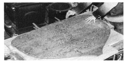
With the glue cured on all of the four pieces making up the transom, the clamps can be removed and a cutting outline can be marked in pencil from a master pattern that Steve has developed for these boats.
