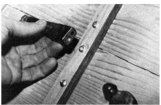
Since the peened-over ends of the rivets will show on the inside of the hull, Steve dresses up their appearance with this tool. It smooths out the surface after peening and gives the rivets a more finished look. Outboard bucking is also required here.
