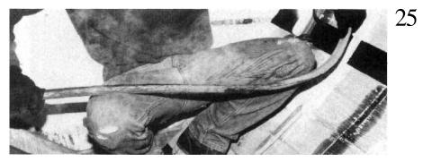
Installation of a bent frame takes place in seconds—it has to, because the wood is only flexible while it's hot, and out of the steambox at room temperature it cools quickly. The first move after pre-bending is to drive the top up behind the sheer clamp, all the while trying to retain its pre-bent shape. This takes some practice, but it's really easier than it sounds.
