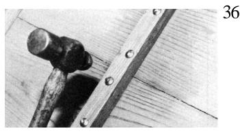
Peening is the next step. A light ball-peen hammer used with many light taps upsets the projecting end and forms it over the burr. Hard blows risk bending the shank inside the wood.
