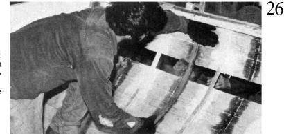
The first clamping takes place down at the heel of the frame near where it bears against the keel. This is where the reverse bend is located, and to get the right amount of curve in it, a fulllength ribband has been temporarily fastened about halfway up in the opening where the new garboard will go.
