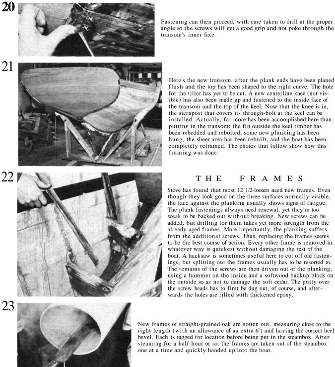
Fastening can then proceed, with care taken to drill at the proper angle so the screws will get a good grip and not poke through the transom's inner face.
