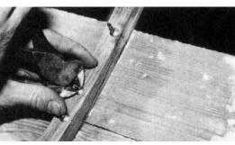
End-nippers cut off the excess length of shank, leaving just enough for peening. Usually about a shank diameter is enough.
