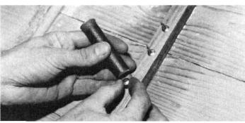
Now for the burrs, or roves, as they're sometimes called. These are a force fit over the rivet shanks, and a short length of round bar with a hole drilled along its axis serves as a tool to drive them on. This tool is used with a hammer on the inside of the boat, while someone bucks up the head of the rivet on the outside using a special iron (see photo #37).
