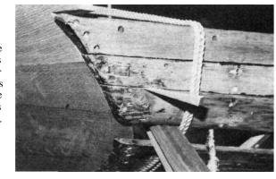
Screw holes in the planking aft, as at the forward end of the boat, have been filled with thickened epoxy, so that new holes may be drilled in optimum locations. The varnished sheer strake, however, is an exception, and in it the old screw holes are reused so as not to change the finished appearance. Before any drilling or fastening is carried out, the planks are wedged as necessary to get seams of even width.
