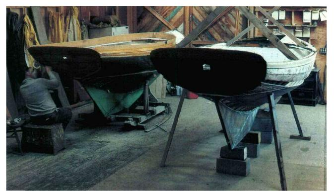
Although there are differences among boats, the first step in a total rebuild usually involves removing the deck, the transom, the stem, and two planks on each side of the boat—the garboard and another plank at the turn of the bilge. The boat shown is approaching that state, and has been blocked high off the floor for access, and braced securely to hold her in shape while the work is going on.
